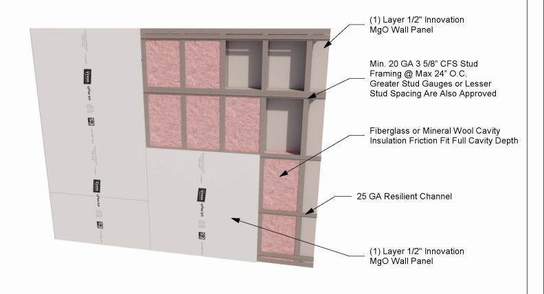
1-HOUR SYMMETRICAL WALL ASSEMBLY 100% LOAD BEARING, STEEL FRAME DESIGN NUMBER:
