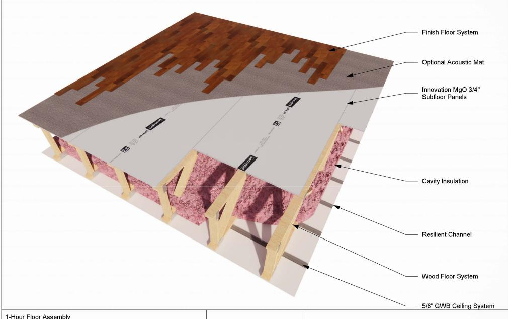
1-Hour Floor Assembly 100% Load Bearing, Wood Frame Design Number:
