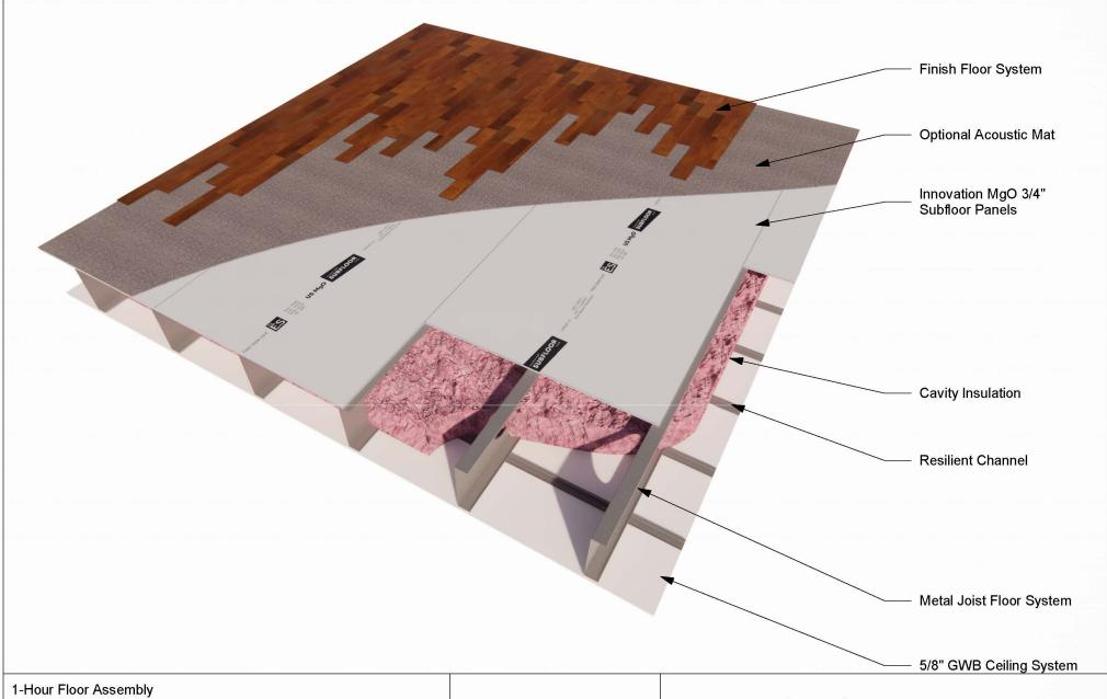
1-Hour Floor Assembly 100% Load Bearing, Metal Frame Design Number:
